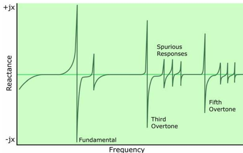
In a quartz crystal resonator, the resistance of a spurious mode can be greater than the main mode resistance or it can be equal to or less than the main mode resistance, depending upon crystal resonator design and processing. A crystal designer has measurable control over the quantity of spurs, the location of the spurs, and the resistance value of the spurious modes.
